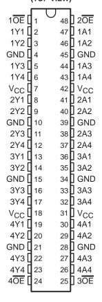
To ensure the high-impedance state during power up or power down,  $\overline{OE}$  should be tied to  $V_{CC}$  through a pullup resistor; the minimum value of the resistor is determined by the current-sinking capability of the driver.
